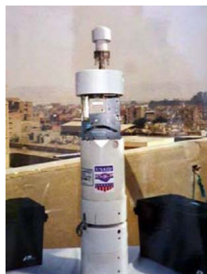
Figure 5.3: The Minivol sampler for PM 10
